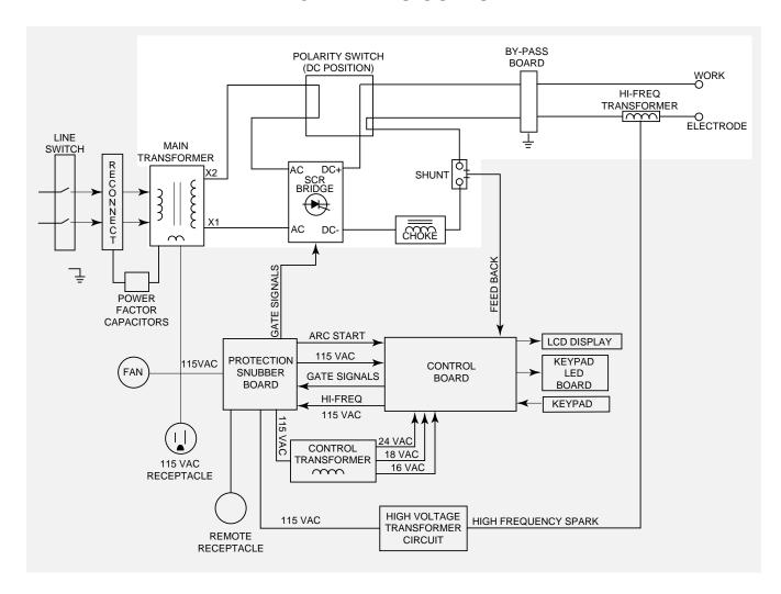
When the polarity switch is placed in either DC position, the AC voltage from the main transformer secondary is applied to the SCR bridge. The SCR bridge and choke circuits are connected in a conventional full wave bridge and filter configuration, resulting in a controlled DC output. Since the choke is in series with the negative leg of the bridge and also in series with the welding load, a filtered DC is applied to the machine's output studs.
